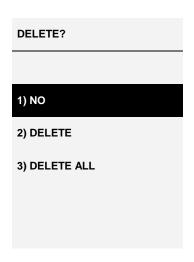
Select the desired delete option with the UP or DOWN arrow keys. If the NO option is selected and then the ENTER key is pressed, the system returns to the memory mask. If the DELETE option is selected and the ENTER key is pressed, the current stored results are deleted and the memory mask is returned to. Selecting the DELETE ALL option and pressing ENTER will delete all stored results and return to the memory mask.
