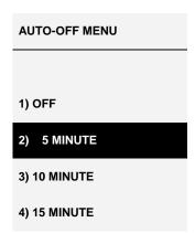
Use the UP or DOWN arrow keys to position the cursor accordingly. Then press ENTER to select the AUTO-OFF function and return to the main menu screen.
