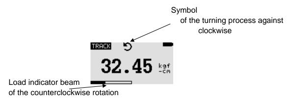
The load indicator bar of the rotation is used to display the load to which the load sensor is exposed.
