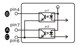
Pins 6 and 7 are switched on after the overload alarm is triggered.
