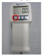
2. When the display shows "0", press the **"UNIT"** button and the **"ZERO"** button simultaneously until **"CAL"** appears on the display.
