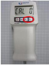
3. After a few seconds the display will show the required **calibration weight**, e.g. 5.00kg for the FK 50 or 10.00kg for the FK 100.
