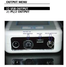
There is an analog output on the device. This generates a signal that goes from +2V to -2V. This signal is a percentage of the maximum value of the force gauge. FOR EXAMPLE..: FL100 50N is measured in the direction of pull, then a -1V signal is applied to the analog output. 75N in compression direction, then + 1.5V is present at the analog output. If the instrument is in PASS - Fail mode, 2V for PASS and 0V for FAIL are present at the analog output.
