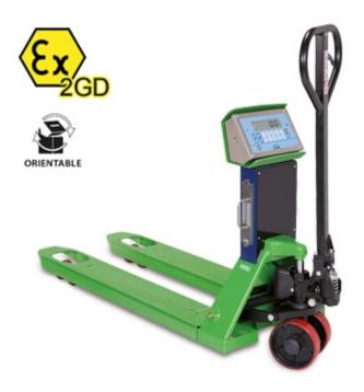
ATEX pallet truck scale for use in hazardous areas (ZONES 1 & 21 & 2 & 22) with Ex II 2G IIB T4 Gb X and Ex II 2D IIIC T197°C Db X protection. Also available in a version approved for legal-for-trade use. Manufactured, calibrated and adjusted in Italy by Dini Argeo, using certified sample weights.
