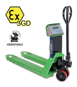
ATEX pallet truck scale for use in areas classified as hazardous (ZONE 2 and 22) with type of protection in accordance with Ex II 3G IIC T6 Gc X and Ex II 3D IIIC T115C° Dc X. Available in approved version for legal-for-trade use. Manufactured, calibrated and adjusted in Italy by Dini Argeo, using certified sample masses.
