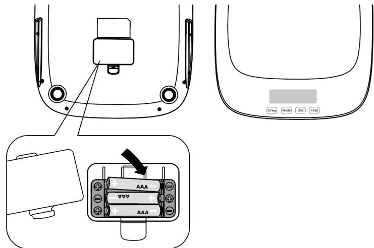
1. Open the battery cover on the underside and insert the batteries. Close the battery cover again.
