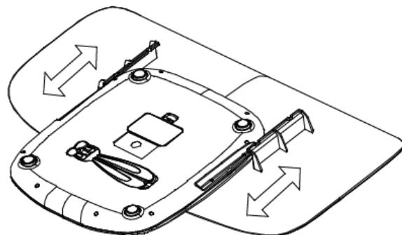
2. Slide the weighing pan over the rails onto the scales so that it engages firmly.
