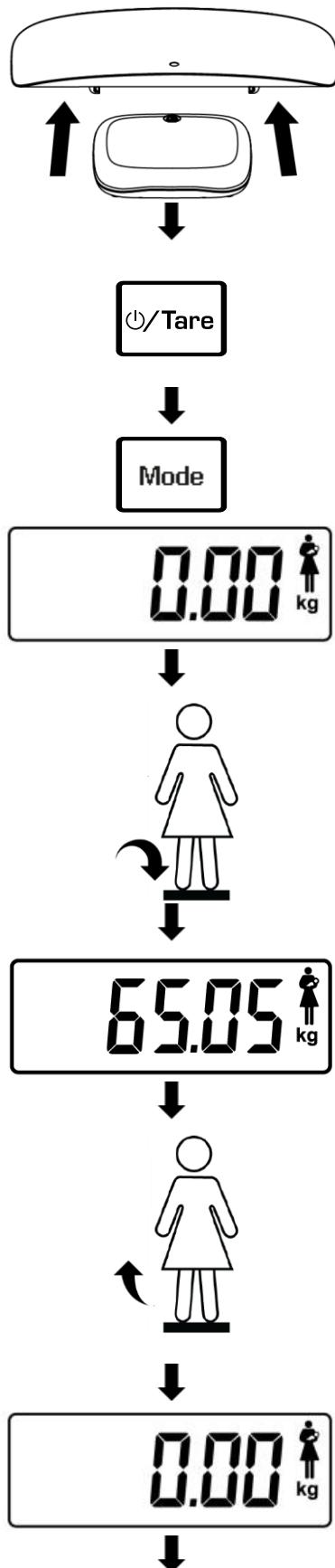
⇒ Remove the weighing pan before switching on the scales.
